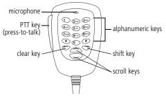
The alphanumeric keys can be used in trunked mode to directly dial any number you can dial using the shift key and scroll keys. In addition, the alphanumeric keys can be used to dial special MPT functions as summarized in the following table. The availability of these functions is dependant on the way your radio is programmed and the way your network operates.
